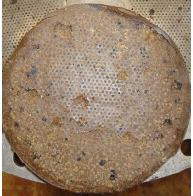
Figure 1. Extreme case of material blocking an extrusion die
