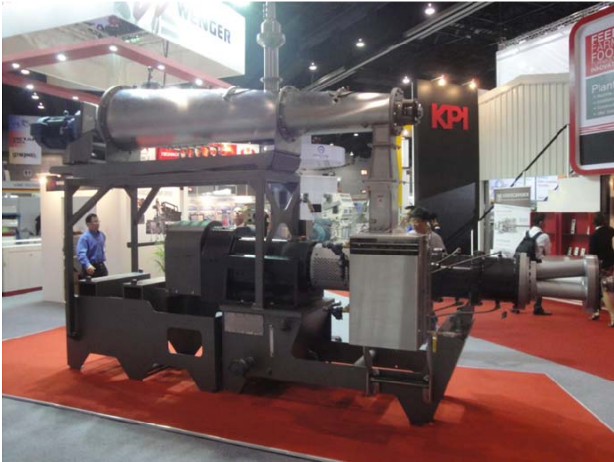
Figure 2. High capacity non parallel twin screw extruder for micro pellets
